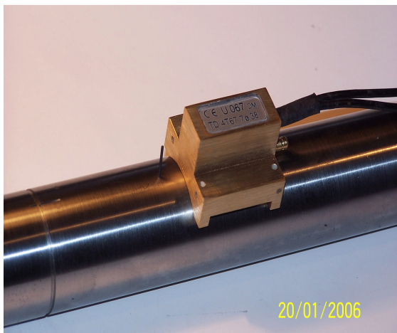
Fig.9 The profiled tandem probe in brass casing
