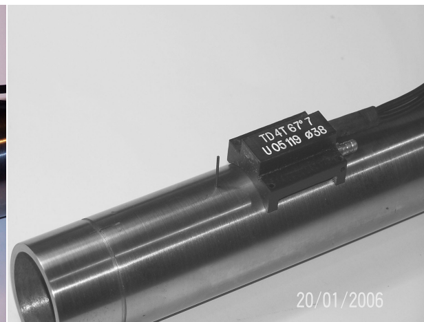
Fig.10 The profiled tandem probe in plastic casing (low profile)
